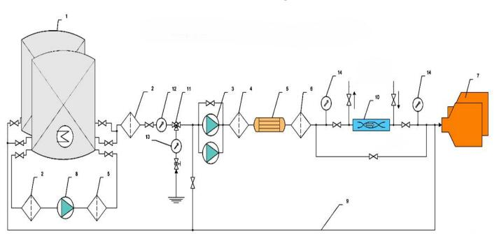
**1.** scheme for installation the TRGA activator for best boiler fuel burning in boiler feed line
