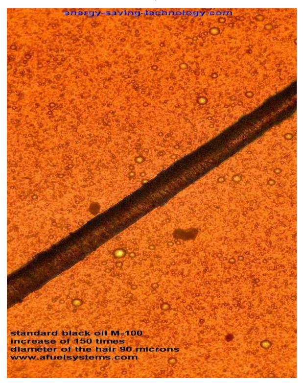
Heavy viscous black oil (M100 type) high-quality, original, water content of 4%, **after treatment** by TRGA homogenizer.
