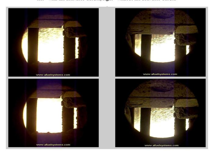
deposits of unburned fuel particles in the boiler, within two months of the boiler – the boiler worked without activator TRGA
